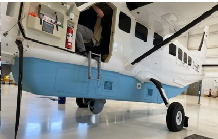
Avcon holds FAA approval, STC SA04744NY, for the Avcon dual lower fuselage mounting system. The Avcon rails provide mounting capabilities for multiple sensors/devices. The FAA approval includes the Avcon vertical lift mechanism for devices/sensors up to 17.7" in diameter within the Avcon Multi-Mission Radome.
