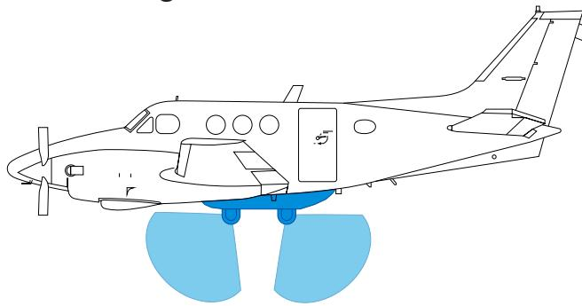
**STC No. SA1746CE** installs structural mounting provisions (ISR Pod) for dual fixed-position sensors such as the Thales I-Master, Wescam MX series (MX-15, MX-15D, MX-20), FLIR Star Safire HD, FLIR Star Safire III, Raytheon Assault TSU QE, Axsys V14HD, UltraForce 350, and others.
